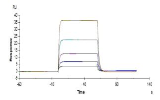
Human CD155, hFc Tag captured on CM5 Chip via Protein A can bind Biotinylated Human DNAM-1, His-Avi Tag with an affinity constant of 264nM as determined in SPR assay (Biacore T200).
